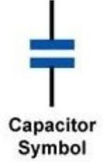
$$1 \text{ Farad} = \frac{1 \text{ Coulomb}}{1 \text{ Volt}} = \frac{3 \times 10^9 \text{ esu of charge}}{\frac{1}{300} \text{ esu of potential}} = 9 \times 10^{11} \text{ esu of Capacitance}$$
