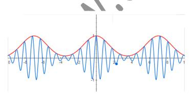
When at least two or more than two waves of slightly different frequency and wavelength superimposes with each other then the amplitude of the resultant wave obtained will propagate in wave manner. The phase velocity of that amplitude wave is called group velocity in wave motion.
