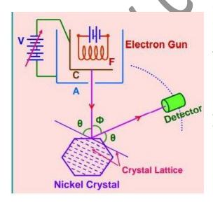
experiment, they have used the electron beam coming from electron gun when the beam is made accelerated by 54 Volt potential drops. After that they allowed that beam to incident on a Ni crystal and get diffraction pattern on the screen when placed in front of that crystal.
