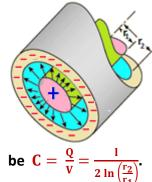
$-\int_{V}^{0} dV = \frac{Q}{2\pi\epsilon_{0}l} \cdot \int_{r_{1}}^{r_{2}} \frac{1}{r} dr \quad Or, V = \frac{Q}{2\pi\epsilon_{0}l} \cdot \ln\left(\frac{r_{2}}{r_{1}}\right) \text{ and finally the capacitance of a cylindrical air capacitor in SI system will be } C = \frac{Q}{V} = \frac{2\pi\epsilon_{0}l}{\ln\left(\frac{r_{2}}{r_{1}}\right)} \cdot \text{Similarly, this capacitance of cylindrical air capacitor in cgs system will Again for cylindrical dielectric capacitor, its capacitance will be$
