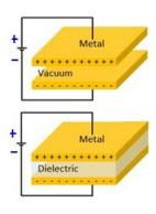
either by air or by dielectric with comparatively separation d. Thus for parallel plate air capacitor, if one plate be charged by positive charge +Q then by electrostatic induction the equal but opposite charge -Q will be induced in the other plate. Here as shown in figure if that other plate be made earthed at zero potential then the effective electric field at any intermediate point P between that two plates will be
