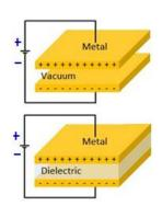
either by air or by dielectric with comparatively separation d. Thus for parallel plate air capacitor, if one plate be charged by positive charge  $+\mathbf{Q}$  then by electrostatic induction the equal but opposite charge  $-\mathbf{Q}$  will be induced in the other plate. Here as shown in figure if that other plate be made earthed at zero potential then the effective electric field at any intermediate point P between that two plates will be
