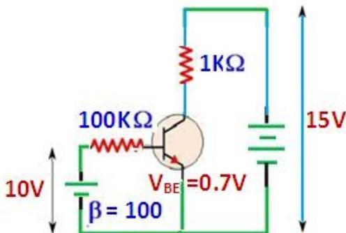
10. A transistor CE circuit is shown in the figure (i) The base current  $I_B$  in mA is (a) 0.093 (b) 0.05 (c) 10 (d) 0.5 (ii) Collector current  $I_C$  in mA is (a) 15 (b) 9.3 (c) 100 (d) 1000
