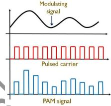
This pulse modulation is used for analog-to-digital conversion.
